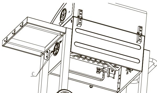
C Vormontierte Schraube M6
